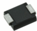
SMCJ9V0CA Fairchild/ON Semiconductor TVS DIODE 9VWM 15.4VC SMC
