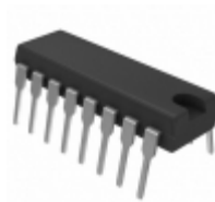
MC10H161PG ON Semiconductor IC DECODER BIN 1:8 16-DIP
