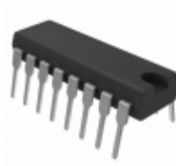
MC10H161P ON Semiconductor IC DECODER BIN 1:8 16-DIP
