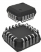
MC10H161FNR2 ON Semiconductor IC DECODER BIN 1:8 20-PLCC
