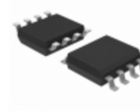
EL5261IS-T7 Intersil IC OPAMP CFA 200MHZ 8SOIC
