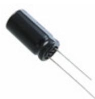
EEU-FS0J512 Panasonic CAP ALUM 5100UF 20% 6.3V T/H
