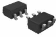
S-1721A1533-M6T1U SII Semiconductor Corporation IC REG LIN 1.5V/3.3V 0.15A SOT23
