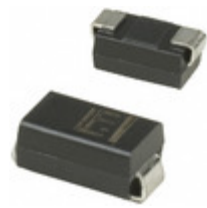
P4SMA170CA Littelfuse Inc. TVS DIODE 145VWM 234VC SMD
