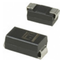
P4SMA170C Littelfuse Inc. TVS DIODE 145VWM 245.7VC SMD
