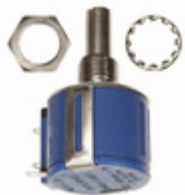
3540S-1-502L Bourns, Inc. POT 5K OHM 2W WIREWOUND LINEAR
