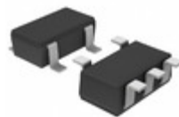
BU34TD3WG-TR Rohm Semiconductor IC REG LDO 3.4V 0.2A 5SSOP
