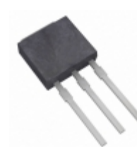
IXTU08N100P IXYS MOSFET N-CH 1000V 8A TO-251
