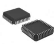
ISPLSI 2032E-110LJ44 Lattice Semiconductor Corporation IC CPLD 32MC 10NS 44PLCC
