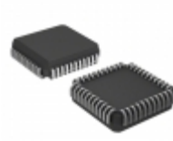
ISPLSI 2032E-135LJ44 Lattice Semiconductor Corporation IC CPLD 32MC 7.5NS 44PLCC
