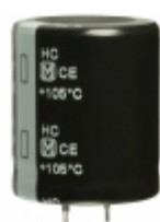
EET-HC2C152DA Panasonic Electronic Components CAP ALUM 1500UF 20% 160V SNAP
