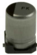
EEV-FK0J220R Panasonic Electronic Components CAP ALUM 22UF 20% 6.3V SMD
