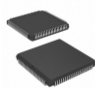
CY37064P84-154JXIT Cypress Semiconductor Corp IC CPLD 64MC 7.5NS 84PLCC
