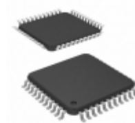
AT87C54X2-RLTUL Microchip Technology IC MCU 8BIT 16KB OTP 44VQFP
