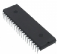
AT87C54X2-3CSUL Microchip Technology IC MCU 8BIT 16KB OTP 40PDIL
