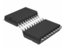
SI88322EC-ISR Energy Micro (Silicon Labs) DGTL ISO 5KV 2CH GEN PURP 20SOIC
