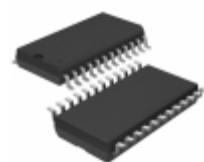
SI88343EC-ISR Energy Micro (Silicon Labs) DGTL ISO 5KV 4CH GEN PURP 24SOIC
