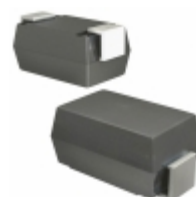
US1G-TP Micro Commercial Co DIODE GEN PURP 400V 1A DO214AC
