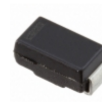
SARS05VR Sanken DIODE GEN PURP 800V 1A SMD
