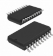
U2794B-MFSG3 Microchip Technology IC DEMODULATR QUAD 1K MHZ 20SSO
