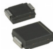
SM30T7.5AY STMicroelectronics TVS DIODE 6.5VWM 11.2VC SMC
