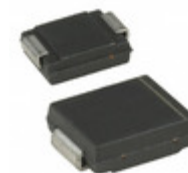
SM30T47AY STMicroelectronics TVS DIODE 40VWM 64.5VC SMC
