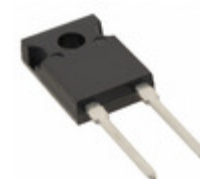
MP915-15.0-1% Caddock Electronics Inc. RES 15 OHM 15W 1% TO126
