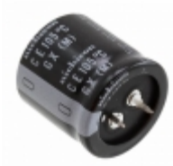
LGX2W181MELB30 Nichicon CAP ALUM 180UF 20% 450V SNAP
