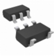
FPF2505 AMI Semiconductor / ON Semiconductor IC LOAD SWITCH FIX CURR SOT23-5
