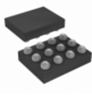
FPF2595UCX AMI Semiconductor / ON Semiconductor IC LOAD SWITCH CURR LIMIT 12WLCS
