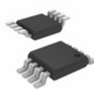
MIC49150-0.9BMM Microchip Technology IC REG LDO 0.9V 1.5A 8MSOP
