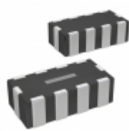
MEA1608PH270T TDK Corporation FILTER LC(PI) 27PF 410MHZ SMD
