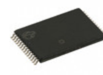
CY62256LL-70ZXI Cypress Semiconductor Corp IC SRAM 256KBIT 70NS 28TSOP
