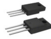
BUL49DFP STMicroelectronics TRANS NPN 450V 5A TO-220FP
