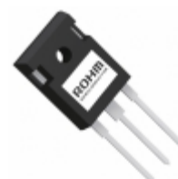
RGT60TS65DGC11 Rohm Semiconductor IGBT 650V 55A 194W TO-247N
