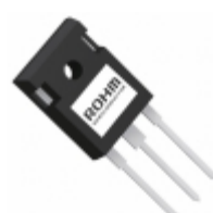
RGT40TS65DGC11 Rohm Semiconductor IGBT 650V 40A 144W TO-247N
