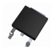
FQD19N10TM_F080 AMI Semiconductor / ON Semiconductor MOSFET N-CH 100V 15.6A DPAK
