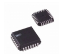
AD767KPZ-REEL Analog Devices Inc. IC DAC 12BIT W/AMP 28-PLCC
