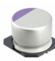
20SVP150M Panasonic Electronic Components CAP ALUM POLY 150UF 20% 20V SMD
