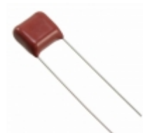
ECQ-E6473RK Panasonic Electronic Components CAP FILM 0.047UF 10% 630VDC RAD
