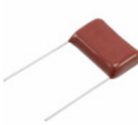
ECQ-E6474KF Panasonic Electronic Components CAP FILM 0.47UF 10% 630VDC RAD
