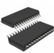
CY8C22345-24PVXAT Cypress Semiconductor Corp IC MCU 8BIT 16KB FLASH 28SSOP
