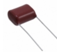
ECW-H6244HC Panasonic CAP FILM 0.24UF 3% 630VDC RADIAL
