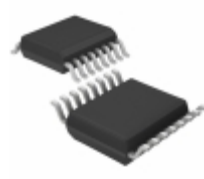
AD5694RBRUZ-RL7 Analog Devices Inc. IC DAC 12BIT I2C QUAD 16TSSOP
