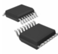
AD5696ARUZ-RL7 Analog Devices Inc. IC DAC 16BIT I2C 4CH 16TSSOP
