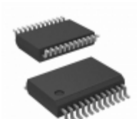
ICL3207ECA-T Intersil IC 5DRVR/3RCVR RS232 3V 24-SSOP
