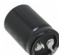
LGN2C471MELY30 Nichicon CAP ALUM 470UF 20% 160V SNAP
