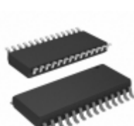
PIC24HJ64GP202-I/SO Microchip Technology IC MCU 16BIT 64KB FLASH 28SOIC
