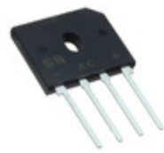
GBU1001HD2G TSC (Taiwan Semiconductor) BRIDGE RECT 1PHASE 50V 10A GBU
