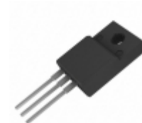
FKPF10N80 Fairchild/ON Semiconductor TRIAC 800V 10A TO220F
