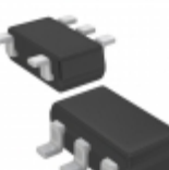
XC6123C641MR-G Torex Semiconductor Ltd IC WATCHDOG TIMER SOT-25
