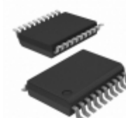
PIC16F18445-I/SS Micrel / Microchip Technology COMPARATOR, DAC, 12-BIT ADCC
