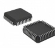
PIC16F874T-20/L Microchip Technology IC MCU 8BIT 7KB FLASH 44PLCC
