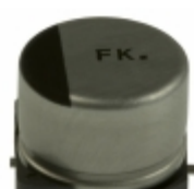
EEE-FK1E221GP Panasonic Electronic Components CAP ALUM 220UF 20% 25V SMD
