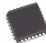
MX574AKEQI+T Maxim Integrated IC ADC 12BIT W/REF 28-PLCC
