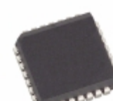
MX574AKP+T Maxim Integrated IC ADC 12BIT W/REF 28-PLCC
