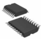
PIC16C716T-20/SO Microchip Technology IC MCU 8BIT 3.5KB OTP 18SOIC
