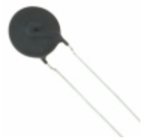
B57237S0220M051 EPCOS ICL 22 OHM 20% 2.8A 15MM
