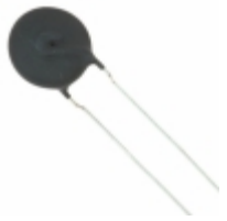
B57237S0330M000 EPCOS ICL 33 OHM 20% 2.5A 15MM
