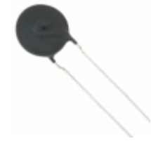
B57237S0150M051 EPCOS ICL 15 OHM 20% 3A 15MM
