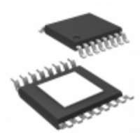
HMC453QS16G Analog Devices Inc. IC PWR AMP MMIC 1.6W 16QSOP
