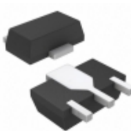
HMC453ST89 Analog Devices Inc. IC MMIC AMP HBT 1.6W SOT-89
