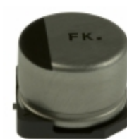
EEE-FK1V151P Panasonic Electronic Components CAP ALUM 150UF 20% 35V SMD
