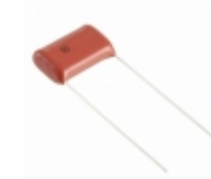
ECQ-E6683RJF Panasonic Electronic Components CAP FILM 0.068UF 5% 630VDC RAD
