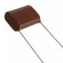
ECQ-E6684JFW Panasonic Electronic Components CAP FILM 0.68UF 5% 630VDC RADIAL
