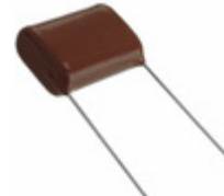
ECQ-E6684KF Panasonic Electronic Components CAP FILM 0.68UF 10% 630VDC RAD
