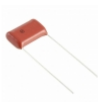
ECQ-E6683RKF Panasonic Electronic Components CAP FILM 0.068UF 10% 630VDC RAD
