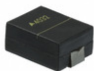
CU4032K275G2K1 EPCOS (TDK) VARISTOR 430V 1.2KA 4032
